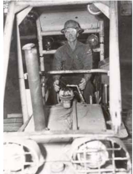
*Fighting fire with a dozer has drastically changed since the Commission purchased it's first unit in 1942. The safety and protection of the dozer operator has greatly improved with personal protective equipment (PPE) and the modified cages on the dozer to prevent debris from entering the cab.*
